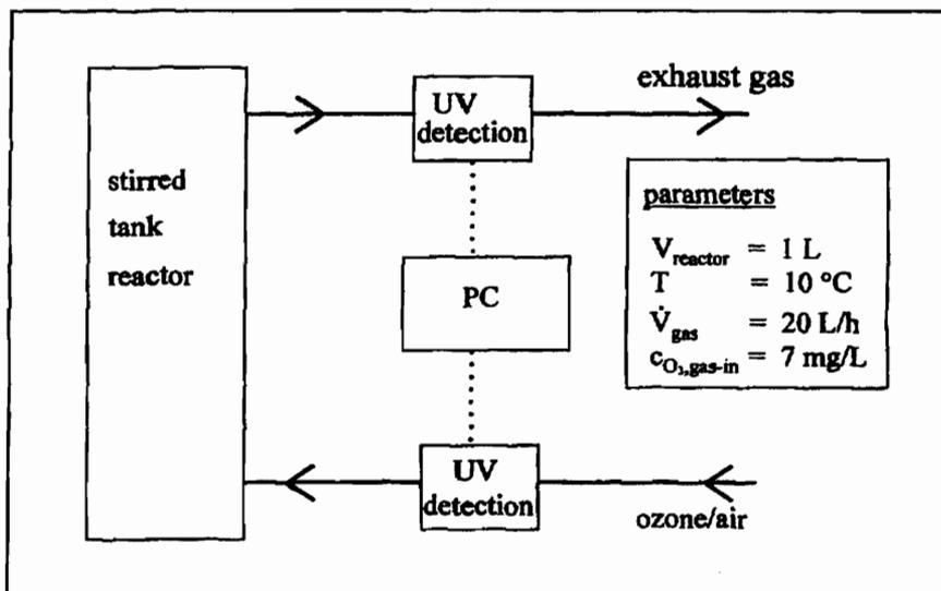
Fig. 1: Apparatus scheme for ozonation.
