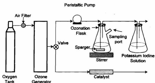
FIGURE 1. Inactivation of microorganisms by ozone; experimental setup (modified from Kim (8)).
