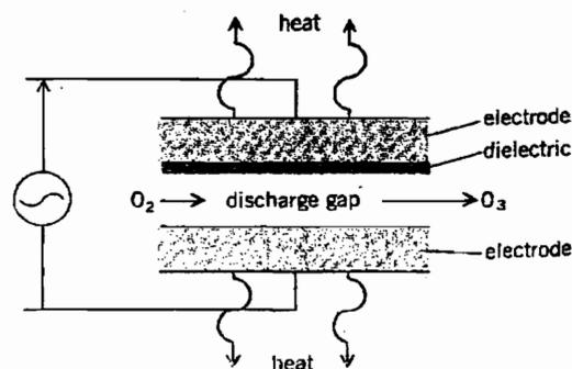
Fig. 1. Diagram of a generic corona cell.
