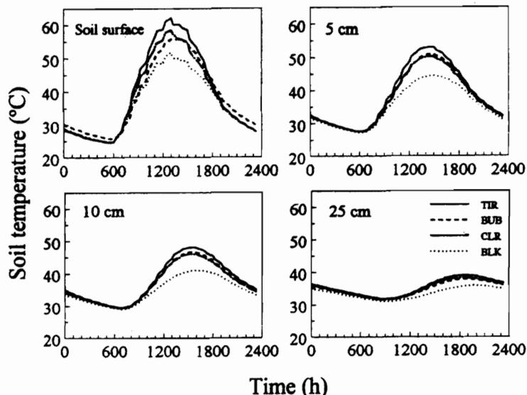
Fig. 2. Diurnal temperature changes measured at four soil depths for four film types at Bradenton, Fla., on a rain-free day (27 July 1996). Polyethylene mulches were: 100 µm thermal-infrared absorbing film (TIR), UV-stabilized bubble film manufactured with two layers of 75 µm-thick polyethylene film (BUB), 30 µm clear low-density polyethylene film (CLR), and 38 µm conventional, embossed black film.
