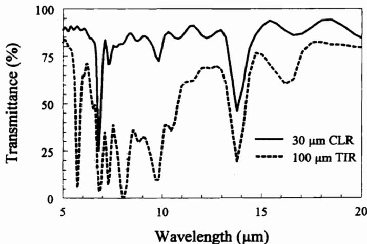
Fig. 1. Comparative transmittance of infrared radiation of a clear, low-density polyethylene film (CLR) vs. a heat-conserving thermal-infrared absorbing film (TIR).
