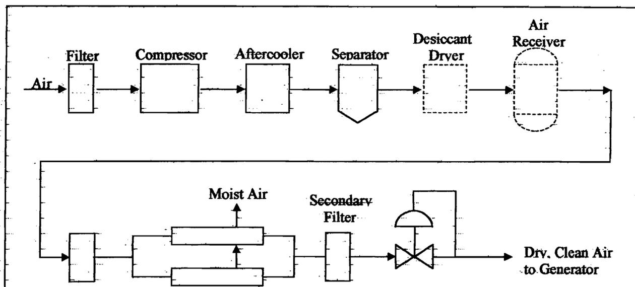
Figure 3-5. Schematic of an Air Preparation System
