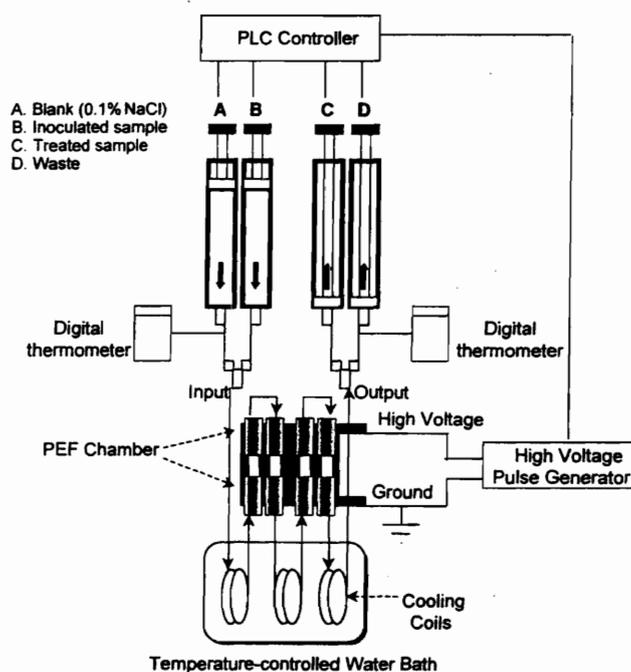
FIGURE 2. PEF bench-scale processing unit and fluid-sample handling system, adapted from the User's Manual of OSU-4C Pulsed Electric Field System and Fluid/Sample Handling Operation (OSU-PEF Team, Food Science and Technology, The Ohio State University, Columbus). Figure is not drawn to scale.
