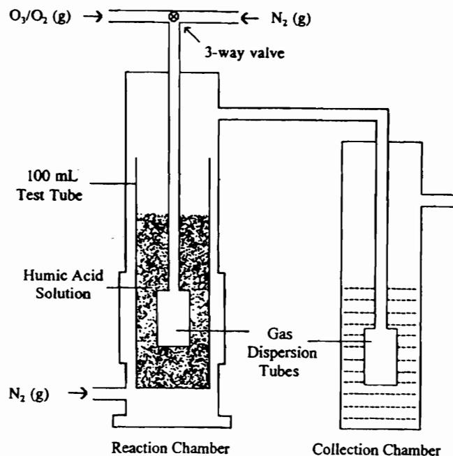
Figure 1. Schematic of the ozonation reaction and collection chambers.
