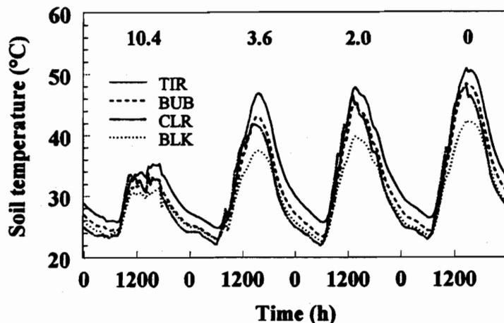
Fig. 3. Effect of rainfall on soil temperatures under four polyethylene mulches at a 5-cm depth at Quincy, Fla., 8 to 11 June 1996. Polyethylene mulches were: 100 µm thermal-infrared absorbing film (TIR), UV-stabilized bubble film manufactured with two layers of 75 µm-thick polyethylene film (BUB), 30 µm clear low-density polyethylene film (CLR), and 30 µm gas-impermeable black film. Numbers above curves indicate rainfall (mm) each day.
